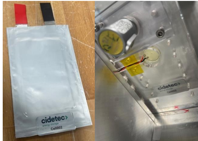
Figure 7: Cell from CIDETEC ID 002 (left), cell pressed with piezo disc (right)
