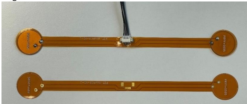
Figure 3: Flex PCB with piezo disc (top) and without (bottom)
